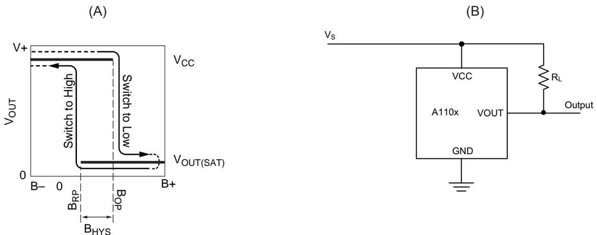
Figure 1. Switching Behavior of Unipolar Switches. On the horizontal axis, the  $B+$  direction indicates increasing south polarity magnetic field strength, and the  $B-$  direction indicates decreasing south polarity field strength (including the case of increasing north polarity). This behavior can be exhibited when using a circuit such as that shown in Panel B.
