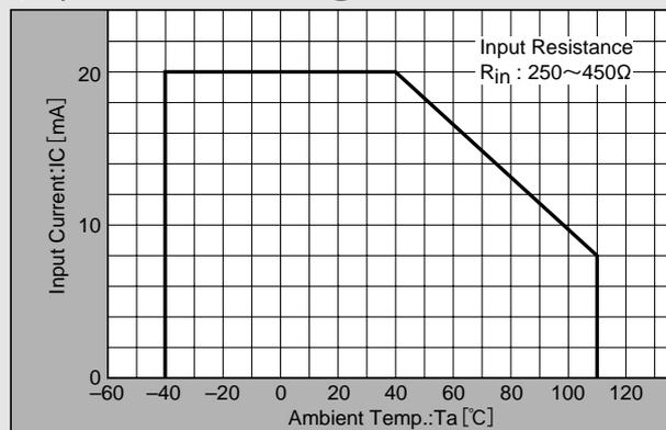
Note :  $R_{in}$  of Hall element decreases rapidly as ambient temperature increases. Ensure compliance with input current derating curve envelope, throughout the operating temperature range.
