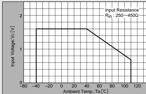
Note : For constant-voltage drive, stay within this input voltage derating curve envelope.
