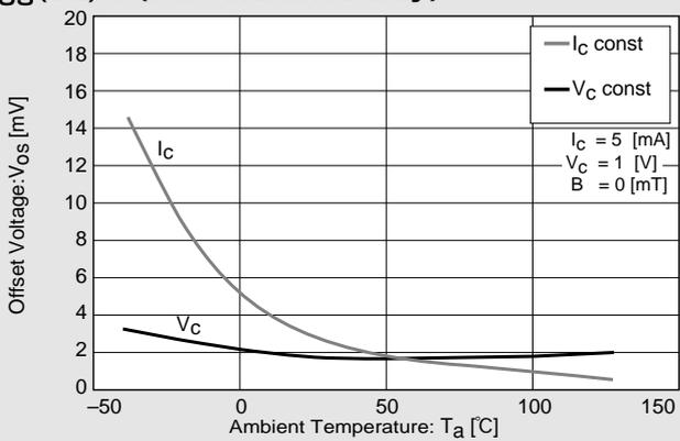
$V_{OS}(V_u)-V_C, V_{OS}(V_u)-I_C$  (For reference only)
