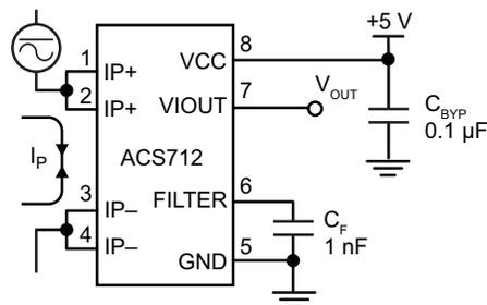
Application 1. The ACS712 outputs an analog signal,  $V_{OUT}$ , that varies linearly with the uni- or bi-directional AC or DC primary sampled current,  $I_P$ , within the range specified.  $C_F$  is recommended for noise management, with values that depend on the application.
