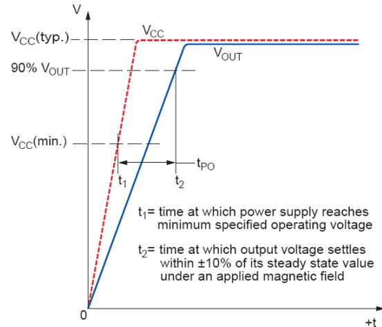
**Rise time ( $t_r$ ).** The time interval between a) when the device reaches 10% of its full scale value, and b) when it reaches 90% of its full scale value. The rise time to a step response is used to derive the bandwidth of the device, in which  $f(-3\text{ dB}) = 0.35/t_r$ . Both  $t_r$  and  $t_{RESPONSE}$  are detrimentally affected by eddy current losses observed in the conductive IC ground plane.
