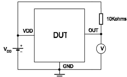
Note 1 -  $B_{OP}$  is determined by putting the device under magnetic field swept from  $E_{RPmin}$  up to  $E_{OPmax}$  until the output is switched on.
