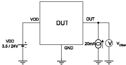
Note 1 - The output saturation voltage  $V_{DS(on)}$  is measured at  $V_{DD} = 3.5V$  and  $V_{DD} = 24V$ .
